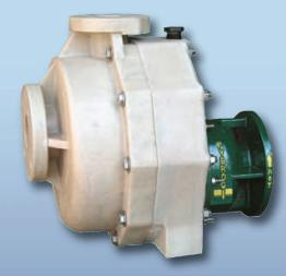
An important feature of the Series 2630 is its replaceable volute extension. The casing volute cutwater in any self-priming pump must be in close proximity to the impeller in order to permit efficient priming. The removable volute extension in the Series 2630 is available in a number of sizes to match specific impeller diameters permitting field hydraulic changes and the restoration of priming efficiency, all without casing modifications or replacement.
